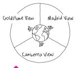
The DSN has three ground stations located approximately 120 degrees apart on Earth (120 + 120 + 120 = 360). This is to ensure that as the Earth rotates, at least one station is able to capture and transmit signals to any deep space mission without any gaps in coverage.
